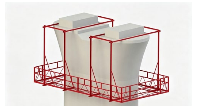
墩顶施工挂篮
